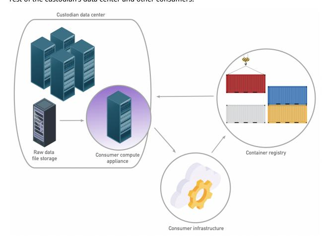
The appliance operates in a locked-down configuration, with access limited to data storage. Rather than simply expose raw files, the appliance packages up the data into industry-standard <a href="DataFrame">DataFrame</a> formats, ready to be consumed by data analytics & machine learning jobs. Each secure network environment exposes the set of DataFrames for their respective consumer.
